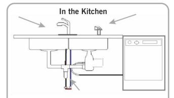
Hoses and water treatment devices may create a potential backflow hazard if not properly isolated with backflow prevention methods.
